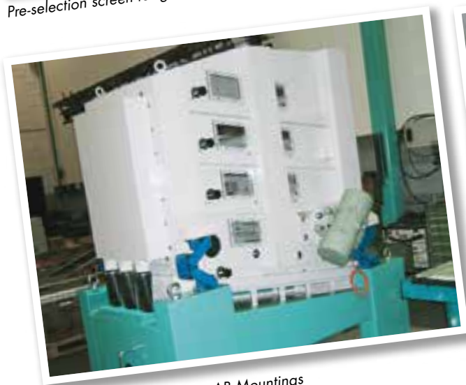
Pre-selection screen for gemstone on AB Mountings
