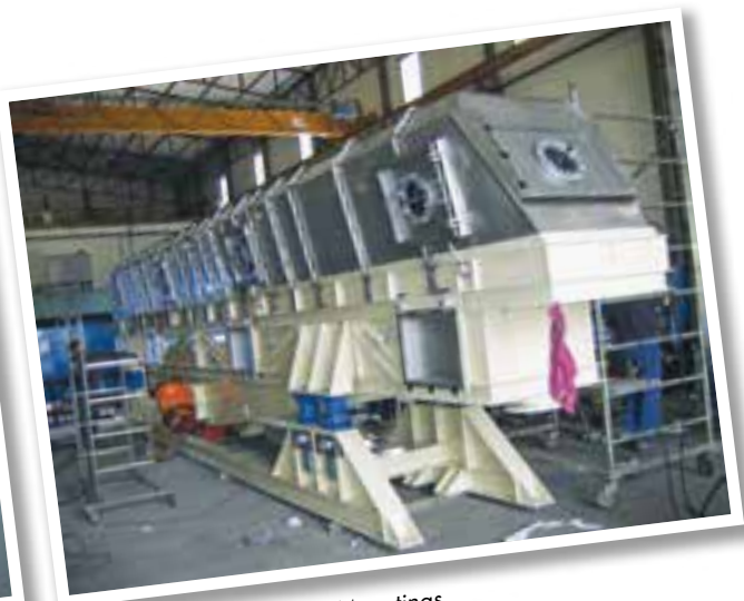
Fluid-bed cooler on AB-D Mountings
