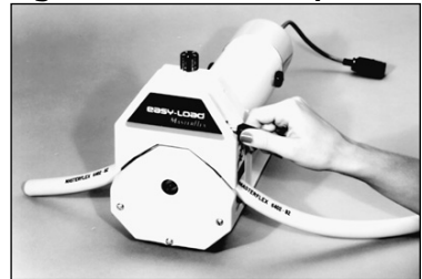
Figure #3. Close Pump
