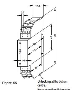
Keep mounting distance to the bottom of 10 mm.
