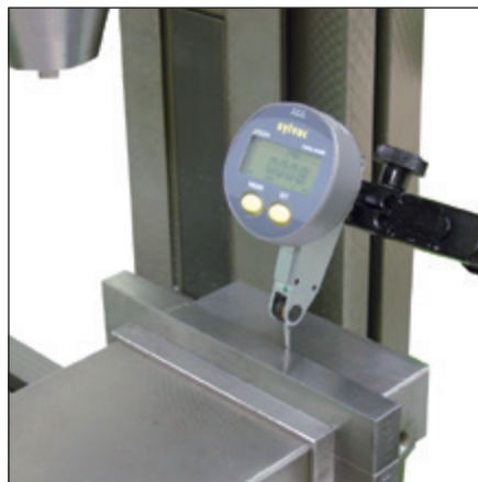
Checking the alignment on milling machine.
