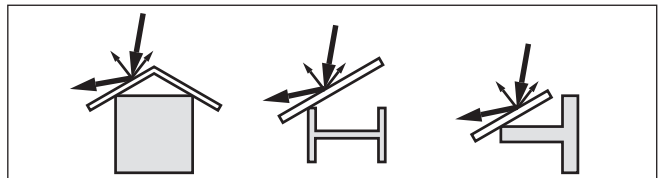
Fig. 17: Cover flat, large-area profiles with deflectors
