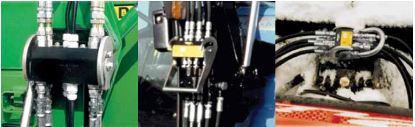
Suitable for quick connection / disconnection of front loaders, and for applications which require the loader tool to be changed
