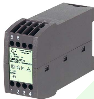
Fig. 1. Transducer SINEAX U 539 in housing P8/35 clipped onto a top-hat rail.
