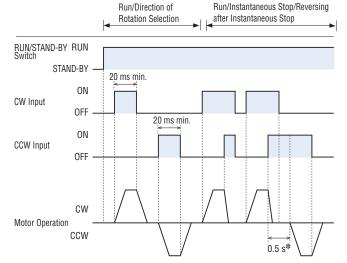
\*Motor does not run for 0.5 s after instantaneous stop, if a reversing run signal is input.
